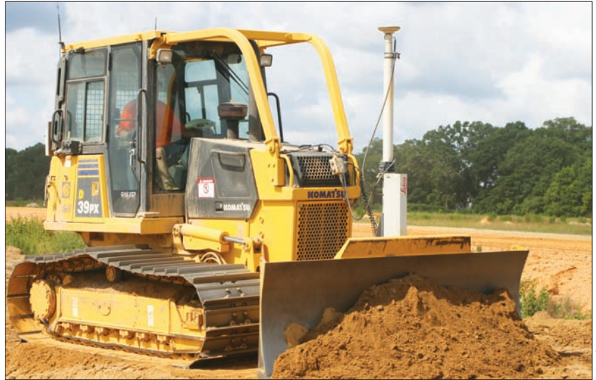
Alan Cawthon fitted this Komatsu D39PX dozer with a GPS system from Leica Geosystems.
