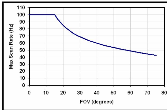
The scan rate is user-selectable from 0 to 100 Hz in 0.1 Hz increments via the graphical user interface. System control software prevents out-of-range inputs for scan rate based on user selection for FOV.
