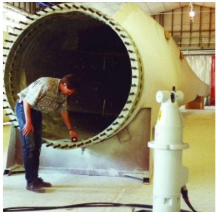
Figure 4: Measurement of the flange area on the rotor blade
