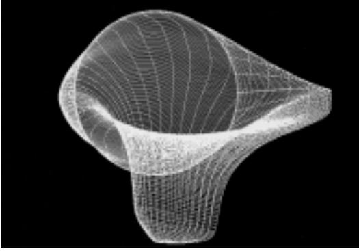
Figure 5: CAD model of the rotor blade
