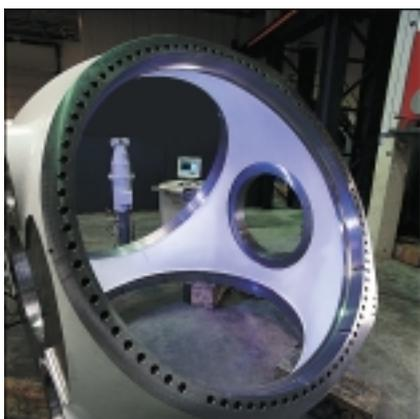
*Figure 9: Dimensional inspection of blade hubs*
