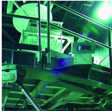
**Leica T-Probe, mounted on the edge of the CDSL platform, lets NASA verify the robots in the MSFC integrated testbed.**
