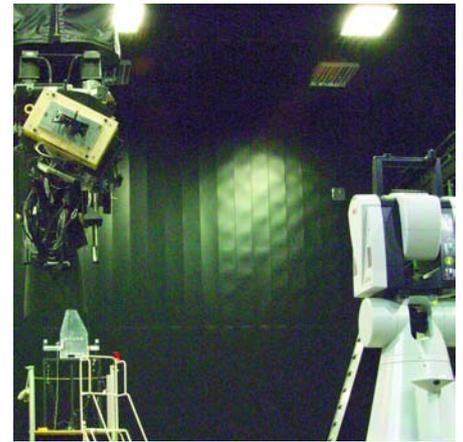
Motion system driven by six hydraulic legs (left); payload section of the Flight Robotics Laboratory (FRL) with the Leica T-Probe mounted and Leica LTD800 Laser Tracker in the foreground (above)
