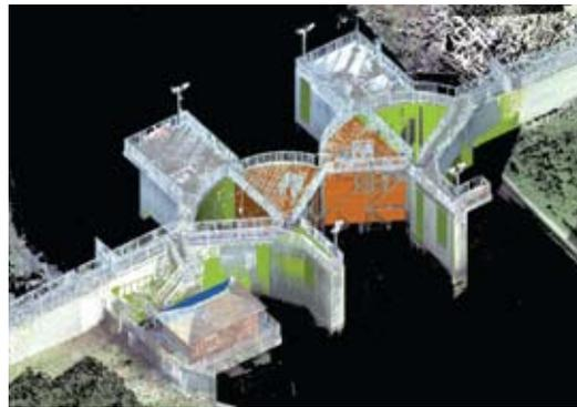
the levee as a baseline and occupied stations at about 100 m intervals to capture the terrain with the ScanStation. This system of intervals created an overlap of data collected, which was registered to create a five-mile point cloud. The result of this combined effort was a six-mile-high density XYZ database.
